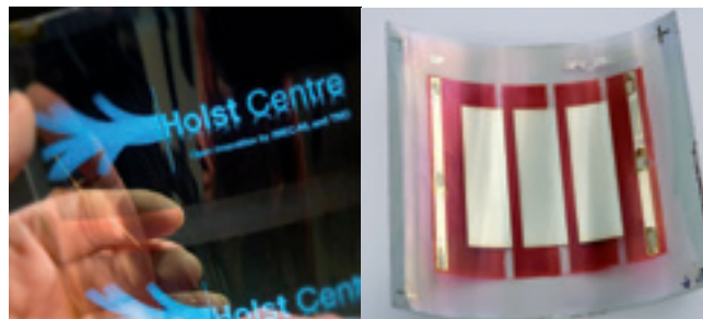
Flexible OLED (left) and OPV device (right)
